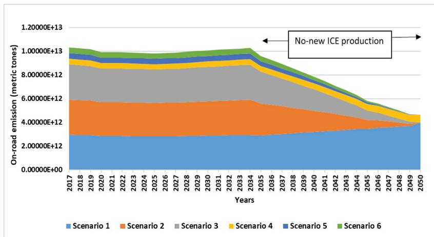
Figure 3: EV adoption impact on on-road CO<sub>2</sub> emission.
